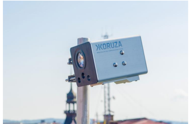
Figure 1: KORUZA the on part of the FSOC link (transmitter).
