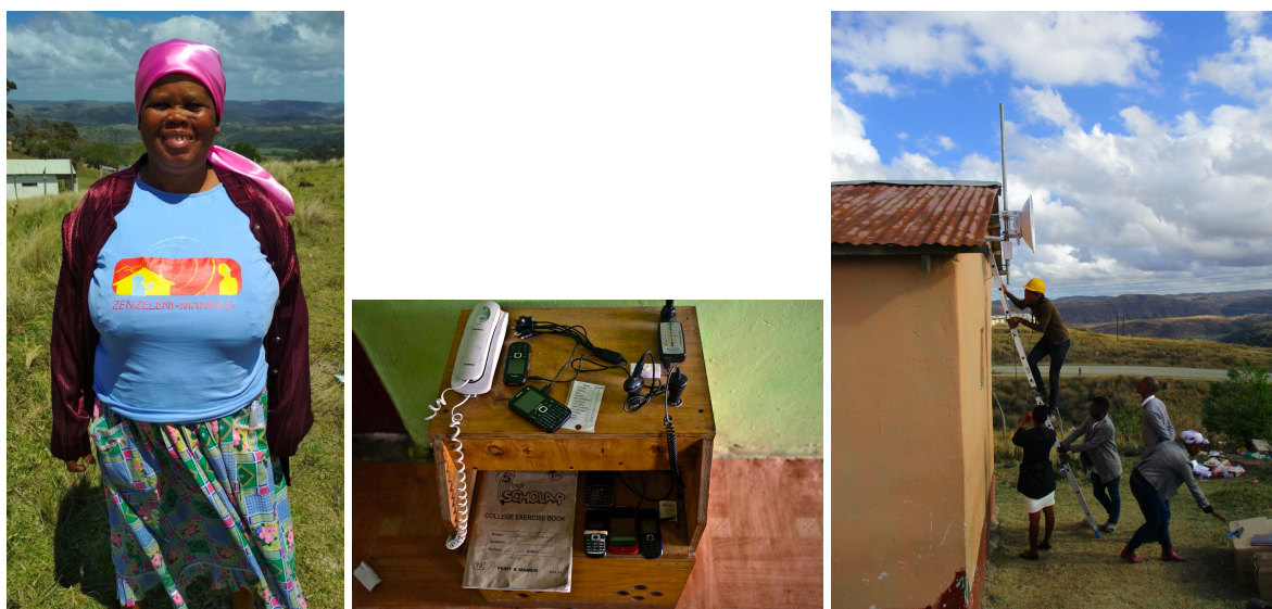
Figure 2: (a) Zenzeleni coop member who sells vouchers, (b) early days internal custom made enclosure housing 2 * 12v deep cycle batteries, a handset plugged directly into a mesh potato with Power over phone line and phone charging apparati; and (c) installing a router and antenna at a residence (this one has a long range throw).
